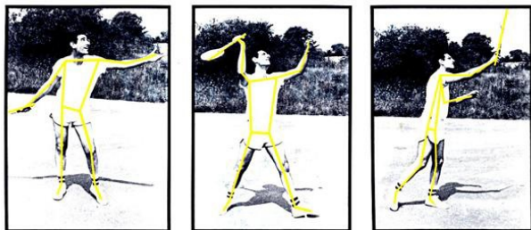
The computer breaks down a beginner's serve into a sequence of stick figures. By comparing a student's stroke with that of a "model" stroke, a teaching pro can make corrections. The computer's stick figures are printed from a high speed camera, and then biomechanical analysis by the computer reveals how the serve can be changed for maximum effectiveness.
