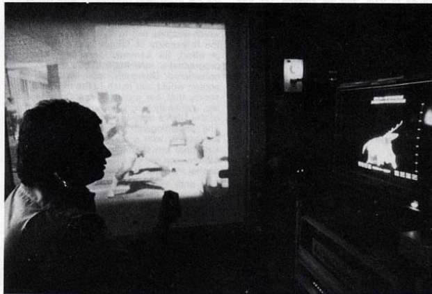
Using an electronic light pen, Dr. Gideon Ariel of the Computerized Biomechanical Analysis company reproduces the movements of the shot putter Al Feuerbach. Simultaneously, this reproduction appears in decomposed images on the television screen and the movements are analysed by the Nova computer which gives a "performance profile" of them. A similar application is used by the United States Olympic Committee on a Data General Eclipse S/250.
