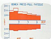
Fatigue curves report the average (solid) and maximum (red line) exercise values for the upstroke and downstroke of each repetition.
