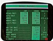
Rehabilitation ratios report, in numerical format, a number of exercise performance values expressed as ratios of performance to body weight, or upstroke to downstroke.
