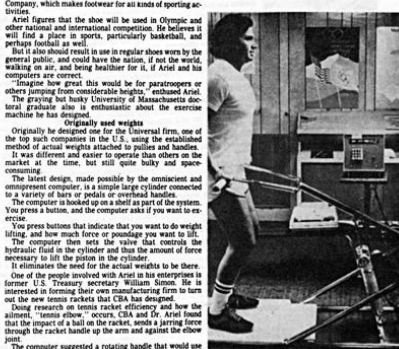
DR. GIDEON ARIEL demonstrates how the computerized exercise machine his Computerized Biomechanical Analysis firm of Amherst designed, with computer operating hydraulic piston to provide the same resistance as weights used on traditional exercise machines. (Richard Carpenter Photo).
