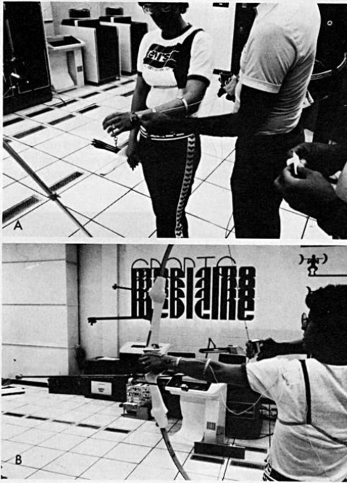
Figure 4. A, The electronic sensor is placed on the wrist of an archer. B, The movements of the bow arm are monitored using the Selspot system (Selcom, Inc., Valdese, North Carolina).
