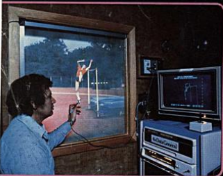
COMPUTER EXPERT Gideon Ariel (above) turns a film into a computer picture. He uses a pen that produces sound. Each time the pen touches a spot on the movie screen, tiny microphones record the pen's position. The computer turns the sound recordings into a stick figure on the computer screen.
