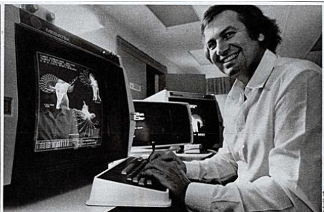
Dr. Gideon Ariel of Computerized Biochemical Analysis Inc. in Amherst, Mass., with his computers that analyze an athlete's fitness or strong points by numerical calculation in a way that can then be visualized on a television screen and studied.
