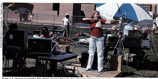
At the U.S. Olympic Committee Elite Athlete Training Program, the computerized biomechanic platform system measures how steadily the archer stands while shooting.
